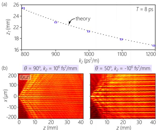
**Fig. 5.** (a) Measured temporal Talbot length  $z_T$  while varying the GVD parameter in the normal regime. The dotted curve is  $z_T = T^2/(\pi|k_2|)$ . (b) Time-averaged intensity  $I(x, z)$  for both normal and anomalous GVD, showing axial invariance despite the underlying temporal evolution (Fig. 3 and Fig. 4).
